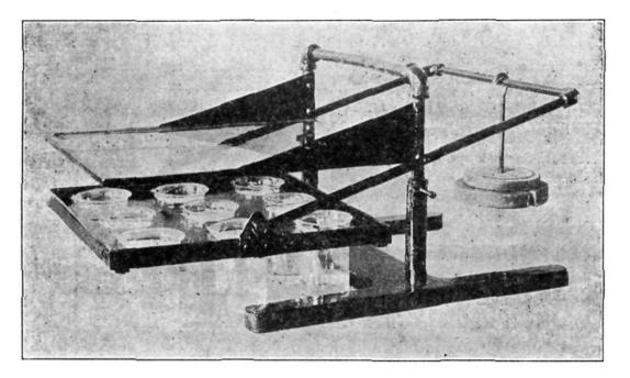
from the source of heat (steam box or electric hot plate) and covered with a glass plate. The evaporations may therefore be made overnight without risk of any of the beakers going dry, and thus a considerable saving of time is effected.
